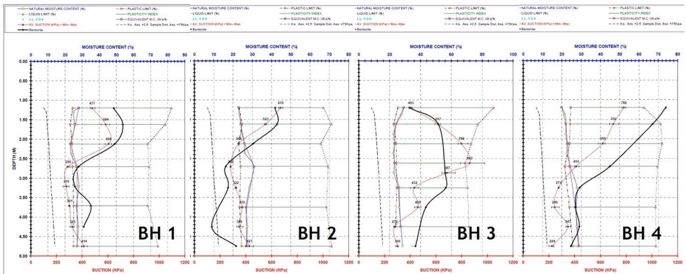
Desiccation evident in all bores to a depth of around 3mtrs bGL with peak suctions of around 600 - 700kPa in BH's 1 & 2, and in the range 600 - 800kPa (BH3) and 700 - 1,100kPa.
