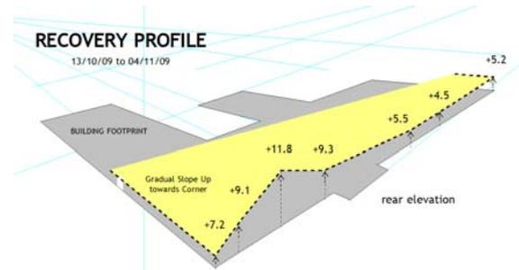
There has been more recovery (11.8mm) in the vicinity of the Wisteria, than elsewhere as can be seen from the image below. There has also been recovery along the side walls of between 5.2 and 7.2mm. Adding the two – the initial distortion and the active movement – gives some feel for the dynamic changes associated with root activity. See graph in adjoining column, below the photograph.
