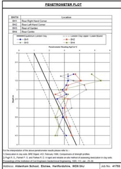
Similar profiles from both tests, with desiccation evident in all bores to a depth of around 3mtrs bGL in the range 0.4 - 0.6 (strains) and 3 - 5Kg/cm<sup>2</sup> (penetrometer)
